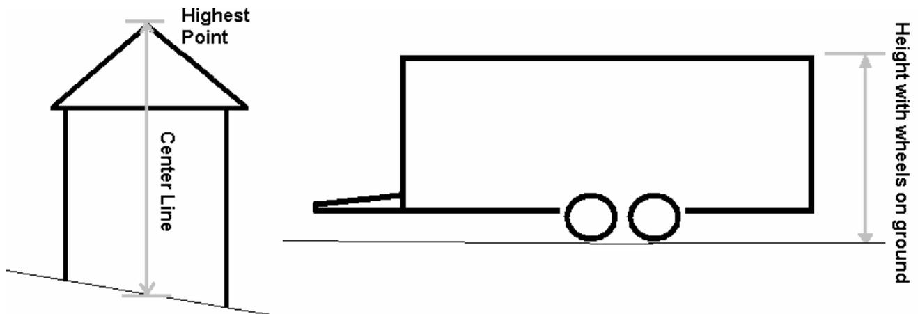
For sheds and other structures constructed on sloping land, the height is the distance between the highest point of the structure and the ground elevation at the centerline of the structure.
